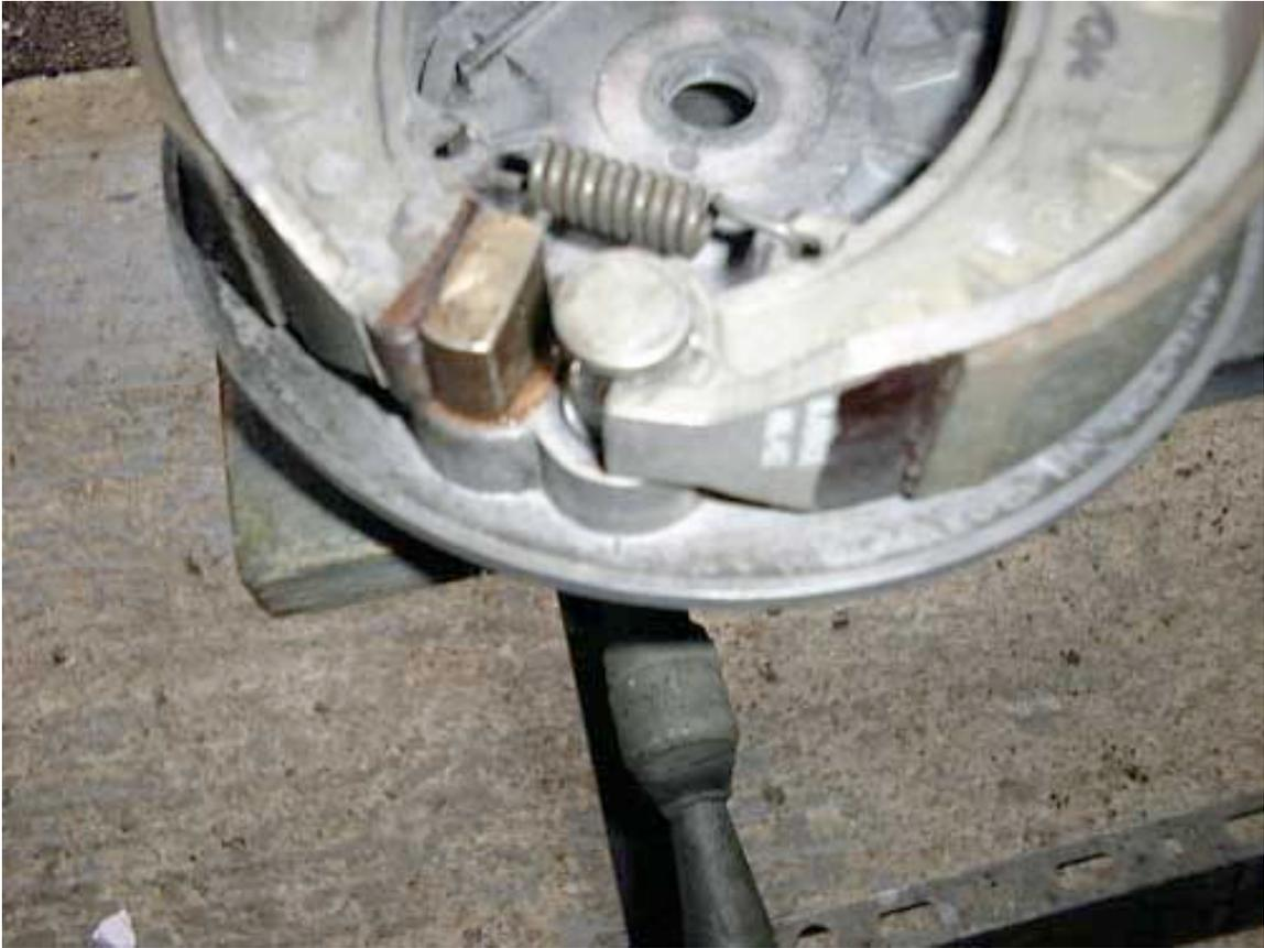
Here the brake is reassembled and fitted back on the motorcycle. Loctite thread lock is useful on all the securing nuts.
