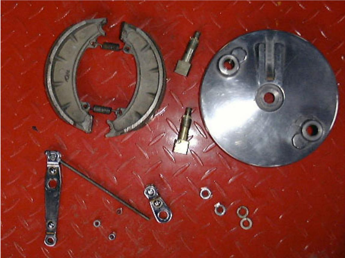
Only a very small amount of grease is needed on the pivot points. The last thing you need is grease on the brake shoes! Not a good idea 😞
