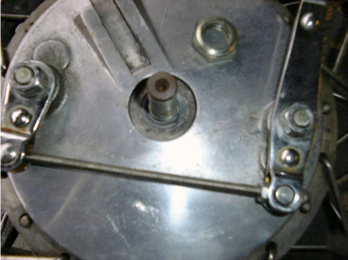
Inside you can see the damage caused by winter riding the Bullet plus trail riding the scrambler. Even after hosing the bike down after each ride, salty water is trapped in the brake drum and causes rapid corrosion.
