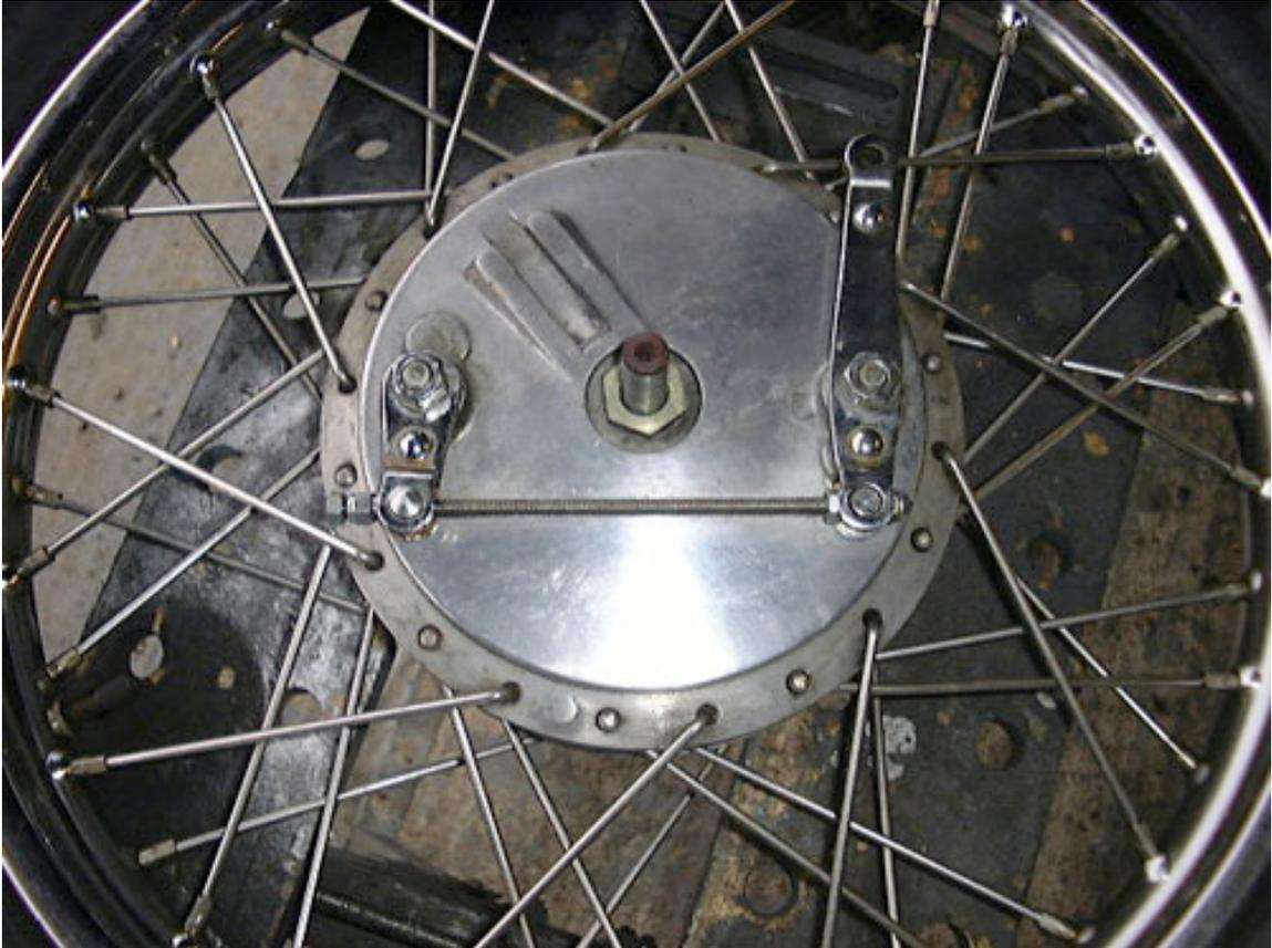
The front brake back plate is held in place with just one central nut.
