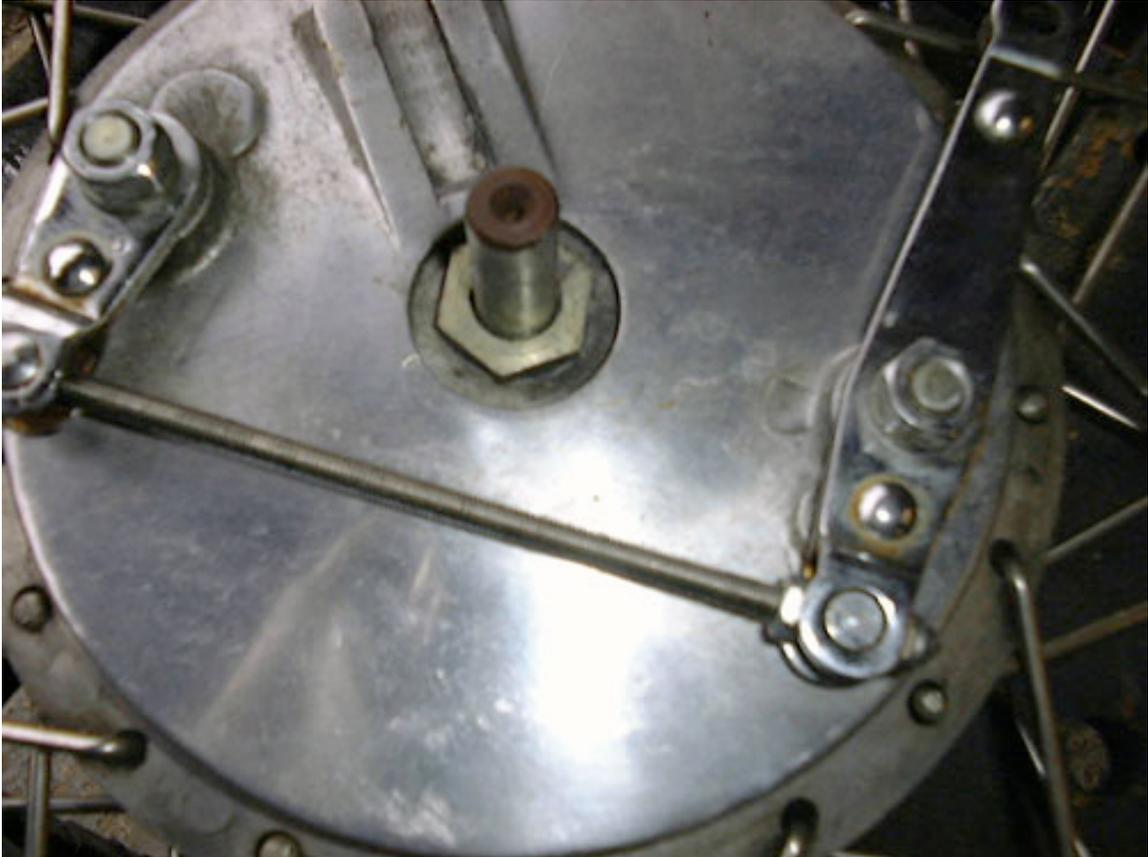
Remove central nut and pull out brake assy.
