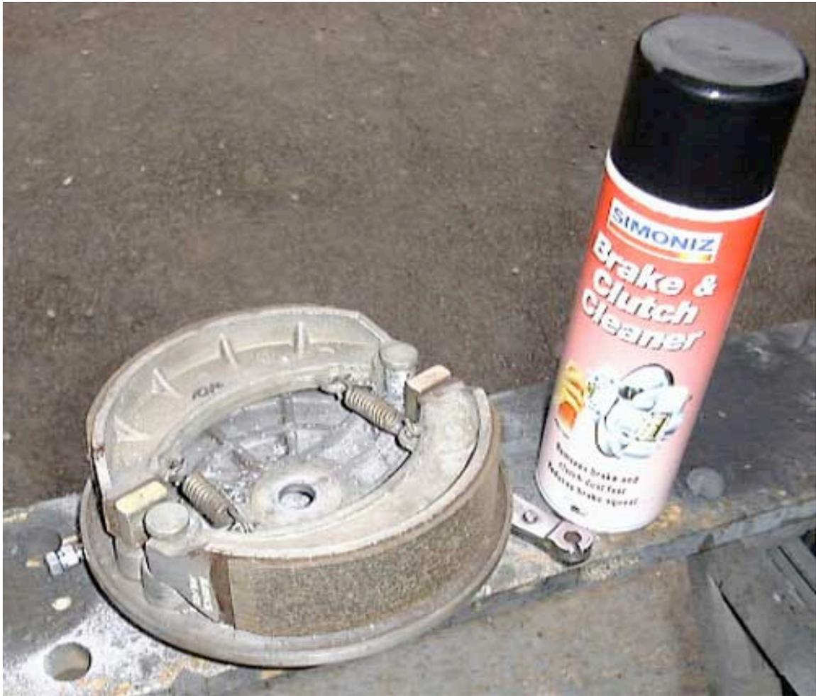
You will need to take the brake shoes off the back plate to clean it thoroughly. This is a good time to replace the shoes with asbestos free items.
