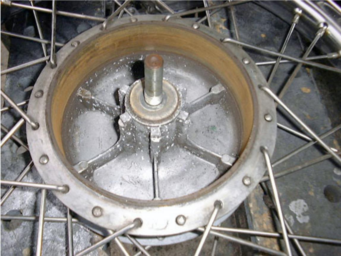
Red rust and white alloy salt damage had rendered the brake unreliable and ineffective.
