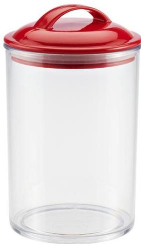
The solution I came up with, is a modified plastic food storage canister from [The Container Store](#), 1.5 qt. Color Pop Acrylic Canister Red Lid, 4-1/2" diam. x 8" h, part number 10059001, for \$13. To accommodate the metal mounting of the ACE Canister, I used a 3" hole saw to remove most of the bottom of the canister and then cut it down to 2-1/4" tall.
