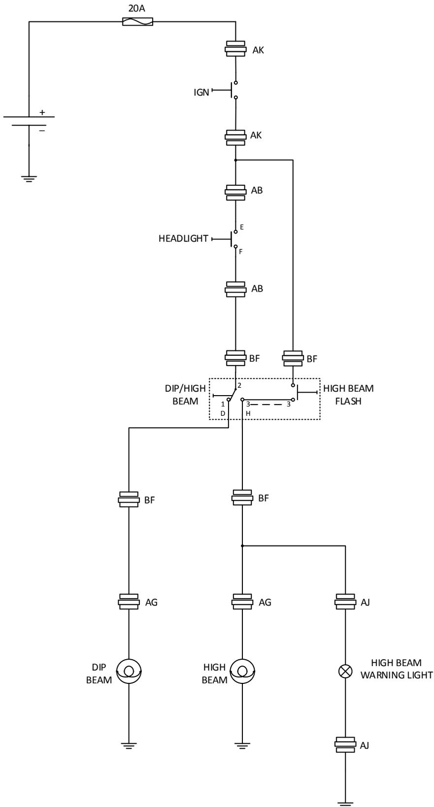
Use in conjunction with the wiring diagram
