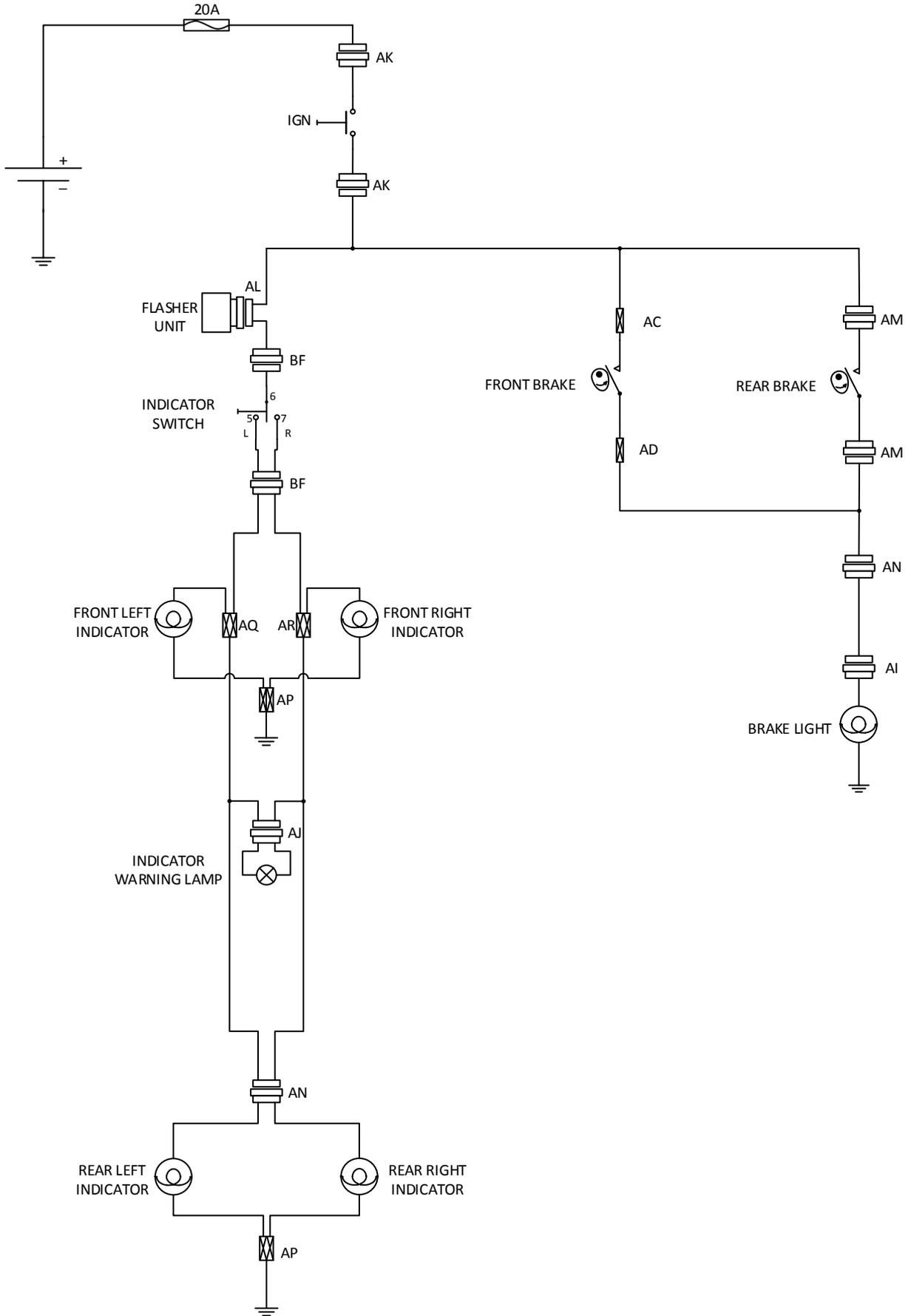
Use in conjunction with the wiring diagram
