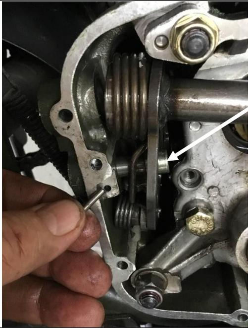
The stop pin also has to be removed. (White arrow).
