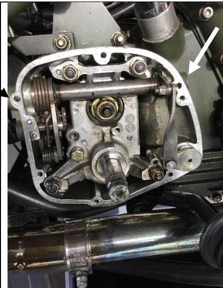
This is the view with the cover off and the kick start spring removed.
